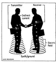
carry data, using a current that is weaker than the and use—NOT a satellite system. natural currents in the body, at speeds comparable with PC modems. Among the possibilities the technology raises are exchanging electronic business cards with a handshake, and paying for goods merely by walking past a scanner. <www.almaden.ibm.com> [End quoting
